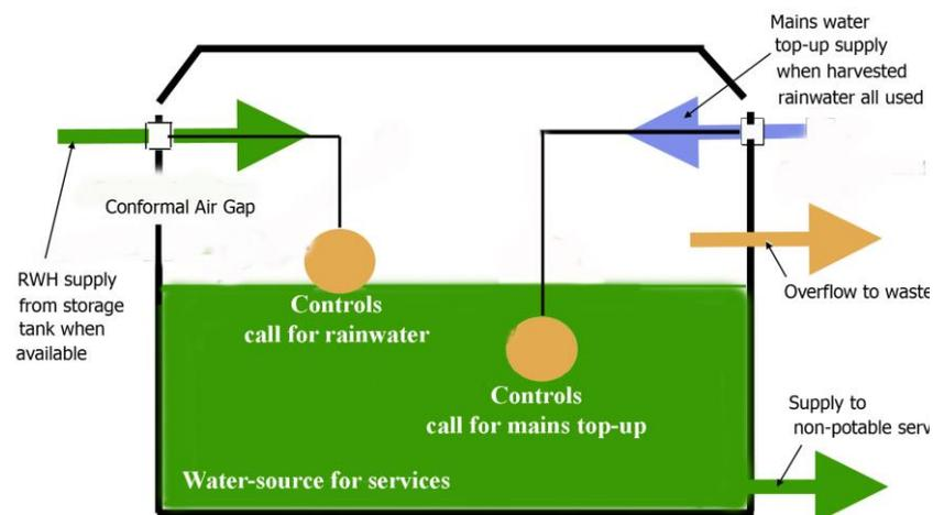
*Schematic showing principles of header-tank operation*
