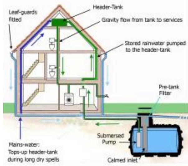
In accordance with the requirements of BS 8515, the water is filtered before entering the storage tank to remove solid particles, usually using a stainless-steel filter installed in the neck of the tank. This filter requires cleaning every 3 months to maintain its efficiency. Failure to do so will possibly lead to progressive clogging of the filter, causing
